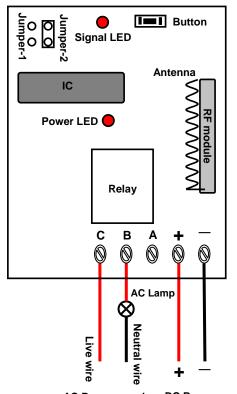
AC Power supply DC Power supply A, B=Normally Closed; B, C=Normally Open.
