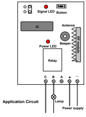
DC0~28V/ AC110~240V A, B=Normally Closed; B, C=Normally Open.
